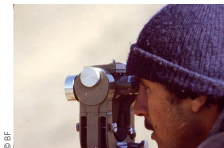
Figure 3. Intersection au théodolite Wild T2, Maroc 1976
